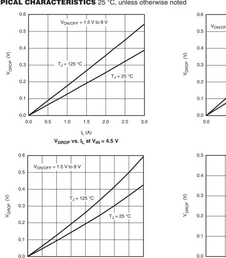
$I_L(A)$  $V_{DROP}$  vs.  $I_L$  at  $V_{IN}$  = 1.8 V
