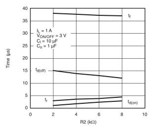
Note: For R2 switching variations with other V<sub>IN</sub>/R1 combinations see Typical Characteristics
