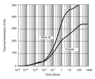
FIGURE 4. Dual SC70-6 Thermal Performance on EVB
