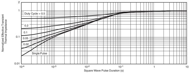
Normalized Thermal Transient Impedance, Junction-to-Foot
