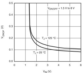
$V_{DROP}$  vs.  $V_{IN}$  at  $I_L = 0.7$  A
