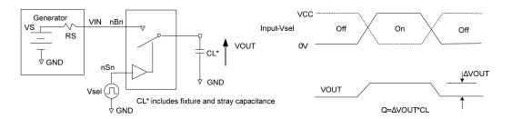
Figure 5. Charge Injection Test
