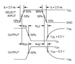
Figure 2. AC Waveforms
