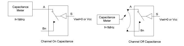
Figure 8. On/Off Capacitance Measurement Setup
