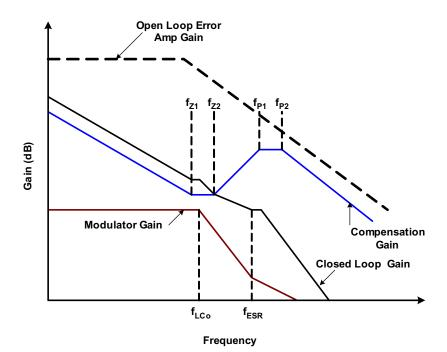
Figure 15. Typical Gain Versus Frequency
