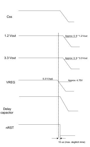
On power up, ALL three regulated supplies, VREG, 3.3 V, and 1.234 V, must be more than 90% of their respective values before the delay timer capacitor on the DELAY pin can start charging.
