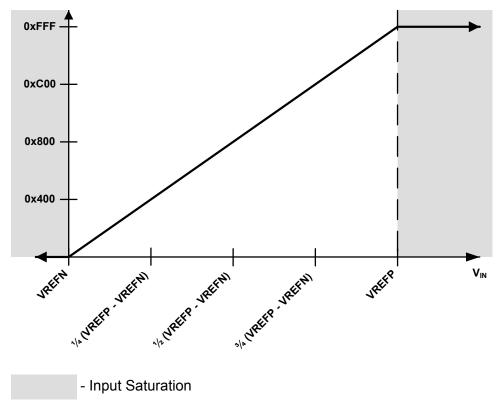
Figure 13-9. ADC Conversion Result
