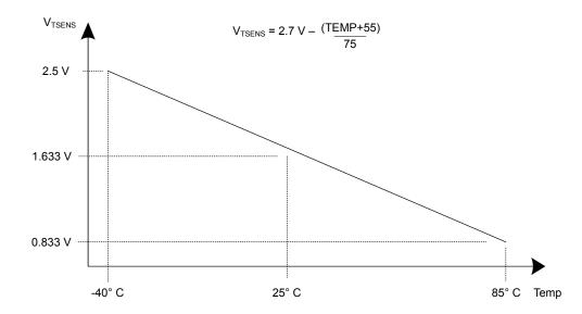
Figure 13-11. Internal Temperature Sensor Characteristic
