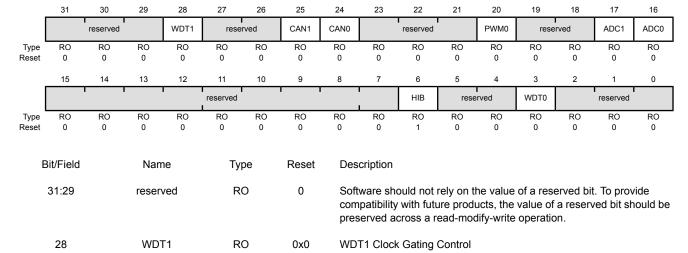
This bit controls the clock gating for the Watchdog Timer module 1. If set, the module receives a clock and functions. Otherwise, the module
