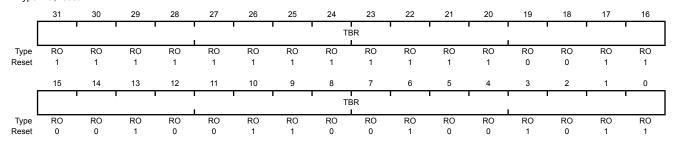
Bit/Field Name Type Reset Description 31:0 **TBR** RO 0x0000.FFFF GPTM Timer B Register
