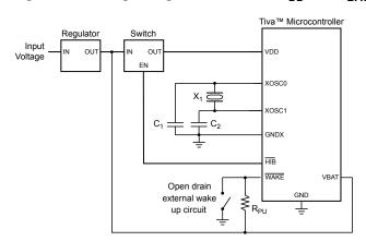
Figure 7-4. Using a Regulator for Both V<sub>DD</sub> and V<sub>BAT</sub>
