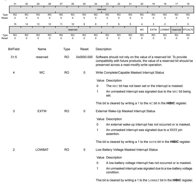
Software should not rely on the value of a reserved bit. To provide compatibility with future products, the value of a reserved bit should be
