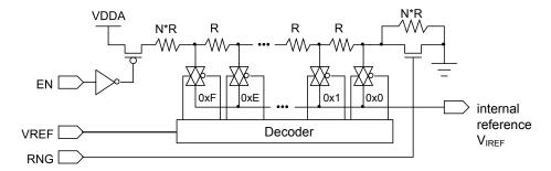
**Note:** In the figure above, N\*R represents a multiple of the R value that produces the results specified in Table 18-2 on page 1090.
