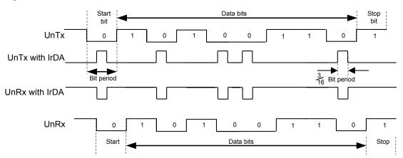
Figure 14-3. IrDA Data Modulation
