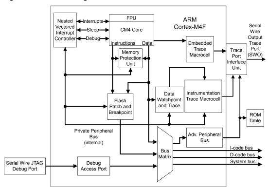
Figure 2-1. CPU Block Diagram
