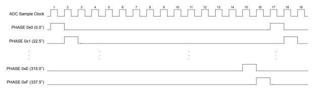
This feature can be used to double the sampling rate of an input. Both ADC module 0 and ADC module 1 can be programmed to sample the same input. ADC module 0 could sample at the standard position (the PHASE field in the **ADCSPC** register is 0x0). ADC module 1 can be configured to sample at 180 (PHASE = 0x8). The two modules can be be synchronized using the GSYNC and SYNCWAIT
