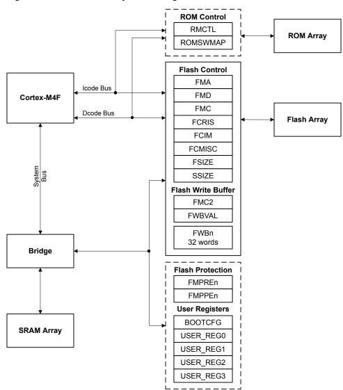
Figure 8-1. Internal Memory Block Diagram
