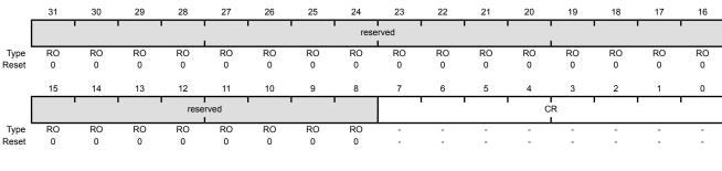
Bit/Field Name Type Reset Description 31:8 RO 0x0000.00 Software should not rely on the value of a reserved bit. To provide reserved compatibility with future products, the value of a reserved bit should be preserved across a read-modify-write operation.
