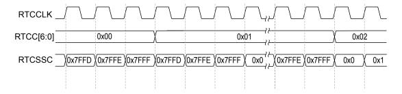
In the case of a trim value below 0x7FFF, the RTCSSC value is advanced from 0x7FFF to the trim value while the RTCC value is incremented from 0x0 to 0x1. If the match value is within that range, the match interrupt is not triggered. For example, as shown in Figure 7-6 on page 488, if the match interrupt was configured with RTCM0=0x1 and RTCSSM=0x2, an interrupt would never be triggered.
