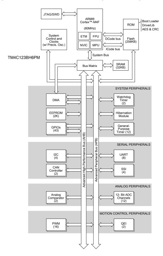
Figure 1-1. Tiva<sup>™</sup> TM4C123BH6PM Microcontroller High-Level Block Diagram
