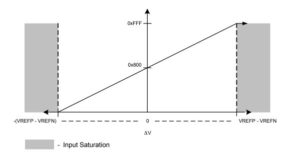
Figure 13-10. Differential Voltage Representation
