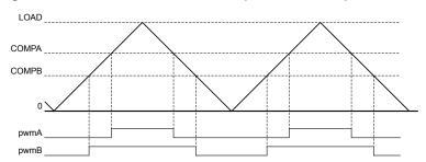
Figure 19-5. PWM Generation Example In Count-Up/Down Mode
