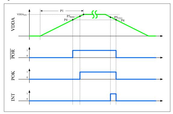
Figure 23-4. Power Assertions versus VDDA Levels
