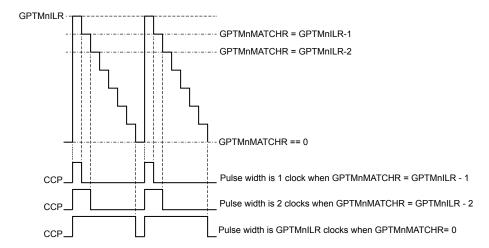
Figure 11-8. CCP Output, GPTMTnILR > GPTMTnMATCHR
