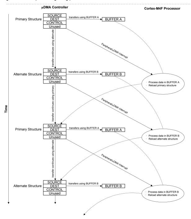
Figure 9-2. Example of Ping-Pong µDMA Transaction
