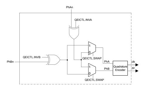
Figure 20-2. QEI Input Signal Logic
