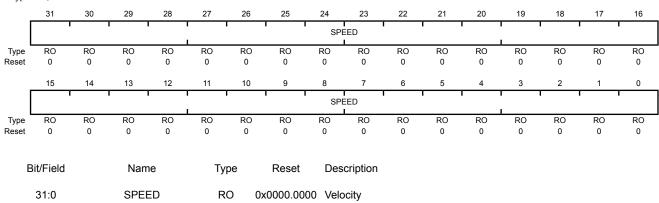
The measured speed of the quadrature encoder in pulses per period.
