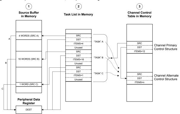
Figure 9-5. Peripheral Scatter-Gather, Setup and Configuration
