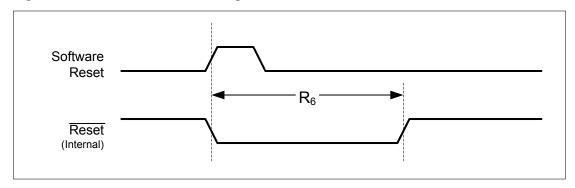
Figure 23-13. Watchdog Reset Timing
