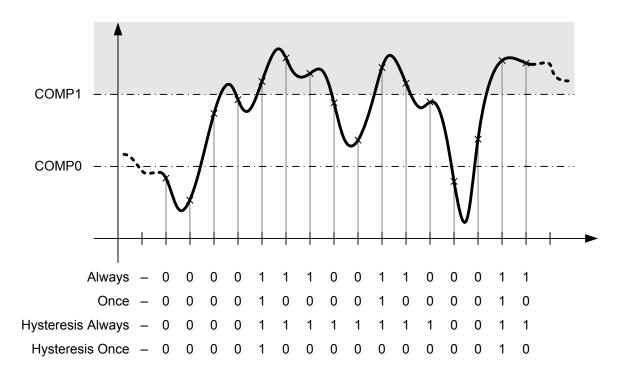
Figure 13-14. High-Band Operation (CIC=0x3 and/or CTC=0x3)
