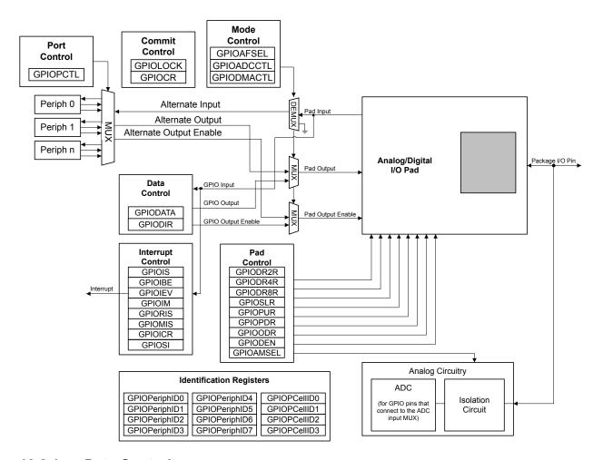
Figure 10-2. Analog/Digital I/O Pads
