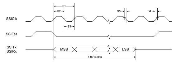
Figure 23-20. SSI Timing for MICROWIRE Frame Format (FRF=10), Single Transfer
