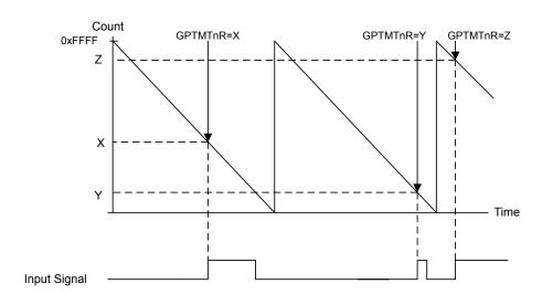
Figure 11-4. 16-Bit Input Edge-Time Mode Example
