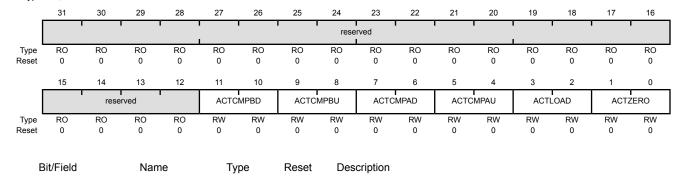
31:12 reserved RO 0x0000.0 Software should not rely on the value of a reserved bit. To provide compatibility with future products, the value of a reserved bit should be preserved across a read-modify-write operation.
