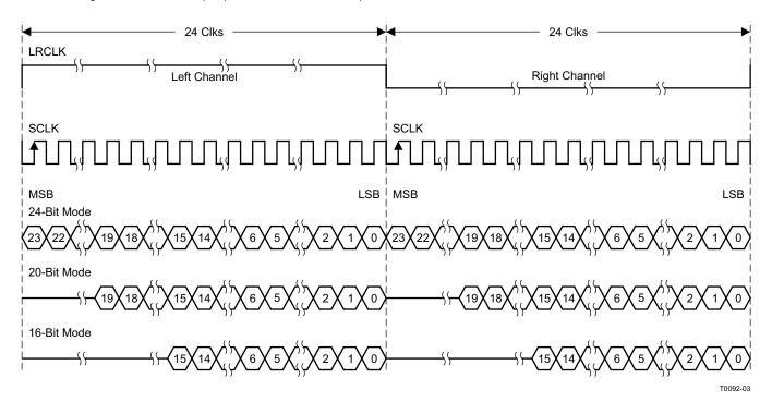
Figure 21. Right-Justified 48-f<sub>S</sub> Bit Format
