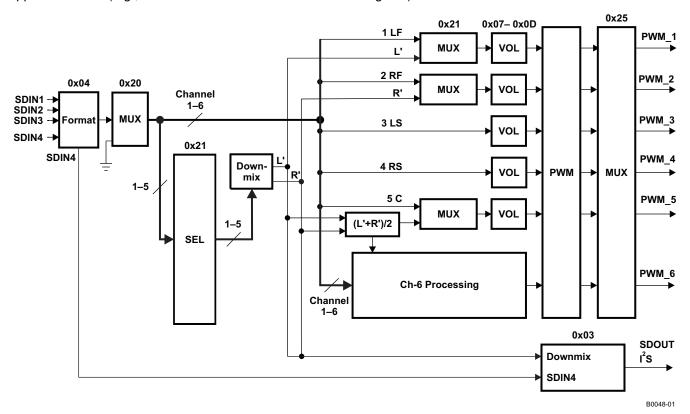
Figure 6. TAS5086 Data Flow Diagram With I<sup>2</sup>C Registers
