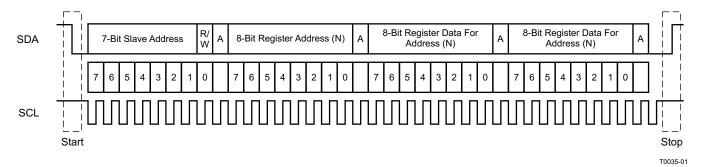
Figure 22. Typical I<sup>2</sup>C Sequence
