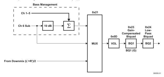
Figure 7. Channel-6 Processing Block Diagram
