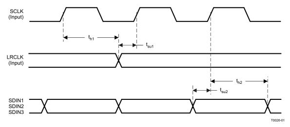
Figure 2. Slave Mode Serial Data Interface Timing
