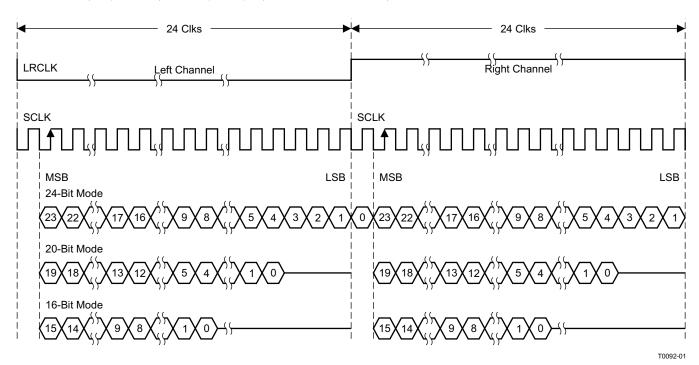
Figure 17. I<sup>2</sup>S 48-f<sub>S</sub> Format
