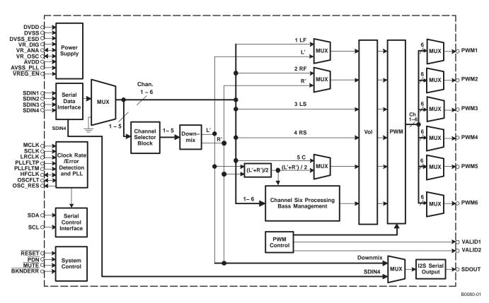
Figure 1. TAS5086 Functional Block Diagram
