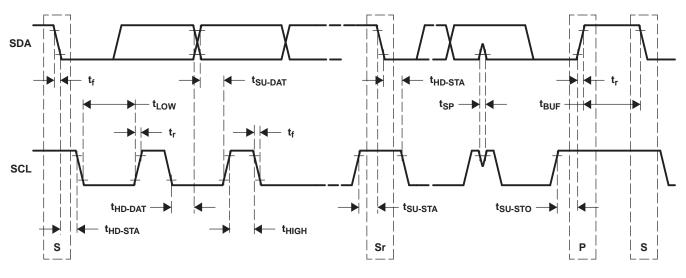
Figure 3. Start and Stop Conditions Timing Waveforms
