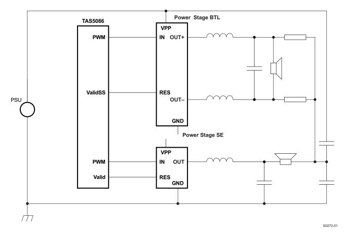
Figure 11. Split-Capacitor Charging With BTL Subwoofer
