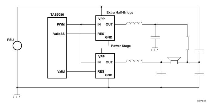
Figure 10. Split-Capacitor Charging With Extra Half-Bridge
