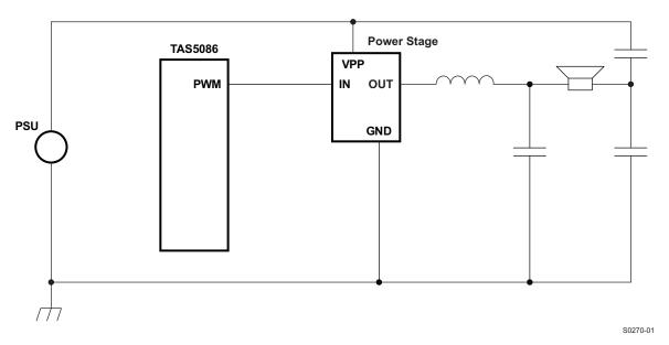
Figure 9. SE Filter Configuration
