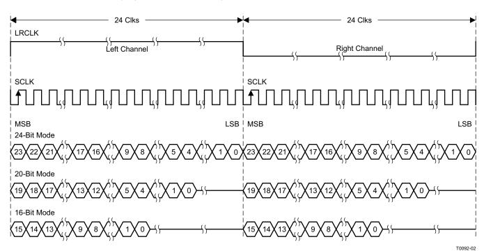
Figure 19. Left-Justified 48-f<sub>S</sub> Format
