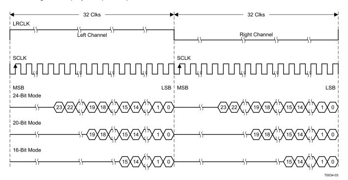
Figure 20. Right-Justified 64-f<sub>S</sub> Format
