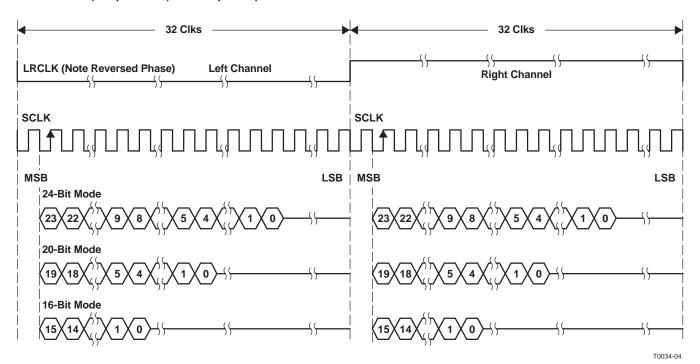
Figure 16. I<sup>2</sup>S 64-f<sub>S</sub> Format
