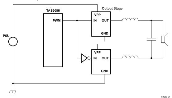
Figure 8. BTL Filter Configuration
