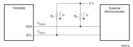
Figure 4. I<sup>2</sup>C Pullup Circuit (With No Series Resistor)
