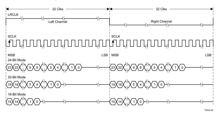
Figure 18. Left-Justified 64-f<sub>S</sub> Format
