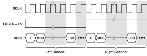
Figure 8. IIS Compatible Serial Format
