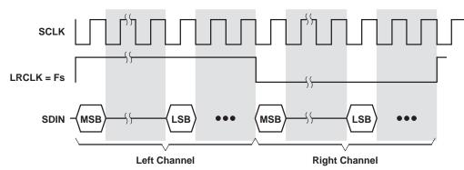
Figure 9. MSB Left-Justified Serial Interface Format
