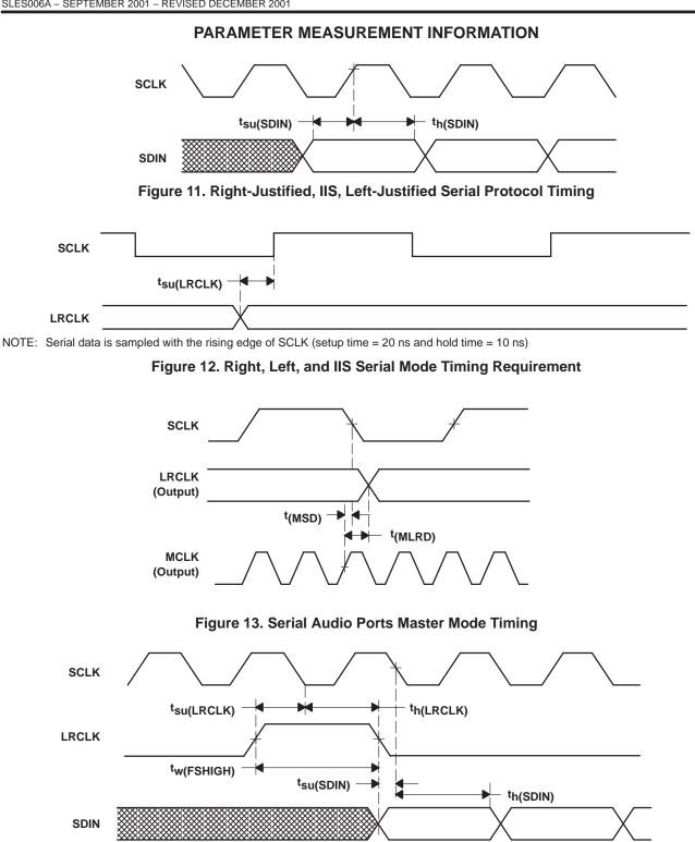
Figure 14. DSP Serial Port Timing
