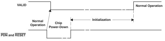
Figure 4. Power-Down Timing
