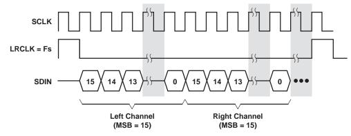
Figure 10. DSP Compatible Serial Interface Format
