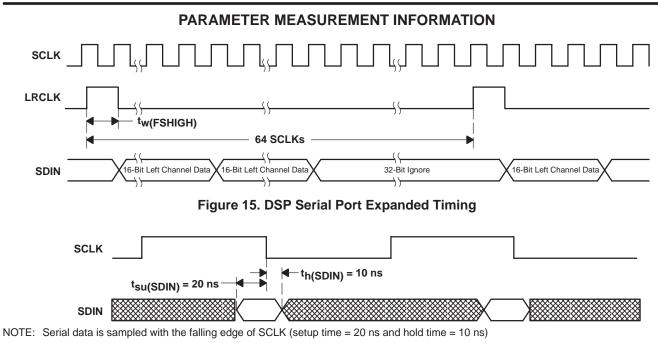
Figure 16. DSP Absolute Timing Requirement
