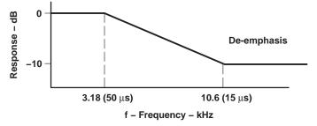
Figure 6. De-Emphasis Filter Characteristics
