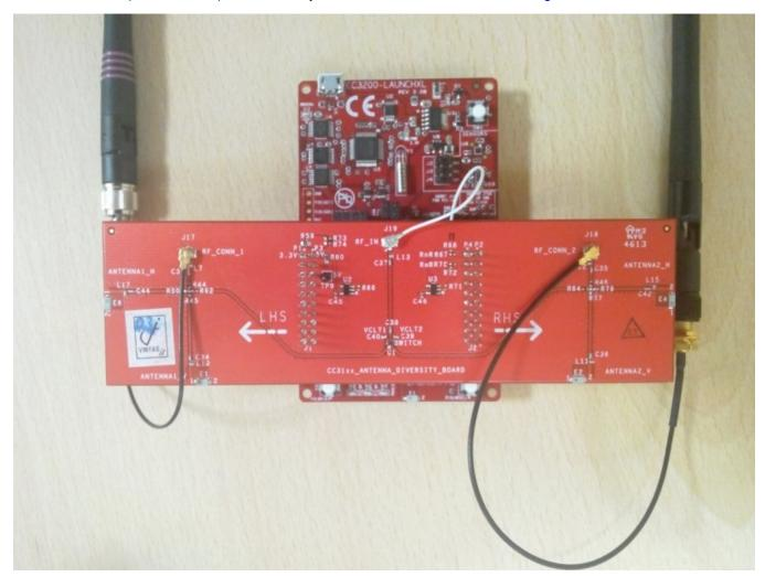
Figure 3-3. Correctly Connected CC3200-LAUNCHXL and CC3ANTENNABOOST Boards
