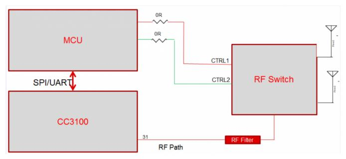
Figure 4-3. Diagram of the Boards' Connections
