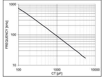
Figure 4. Oscillator frequency vs. C<sub>T</sub> (RT1 = 10k, RT2 = 4.32k)
