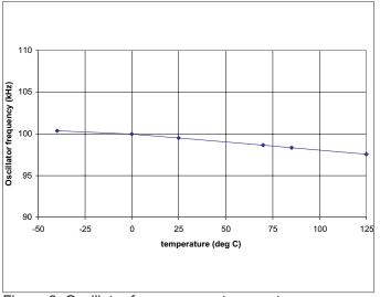
Figure 8. Oscillator frequency vs. temperature.
