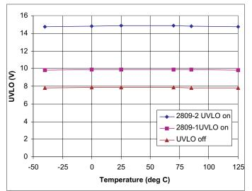
Figure 7. UVLO vs. temperature.
