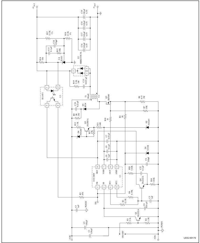
Figure 1. Isolated 50W flyback converter utilizing the UCC3809. The switching frequency is 70kHz, Vin = -32V to -72V, Vout = +5V, lout = 0A to 10A
