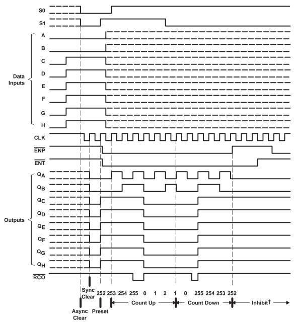
$+\overline{\text{ENT}}$  and  $\overline{\text{ENP}}$  both must be low for counting to occur.
