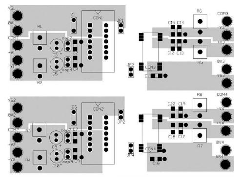
Figure 38. PCB Layout Example, Component-Side View
