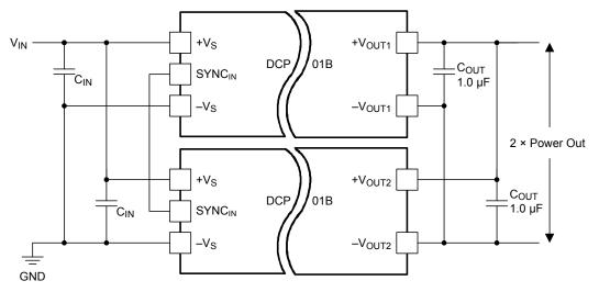
Figure 31. Multiple DCP01B Devices Connected in Parallel
