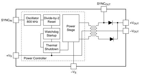
Figure 27. Single Output Device
