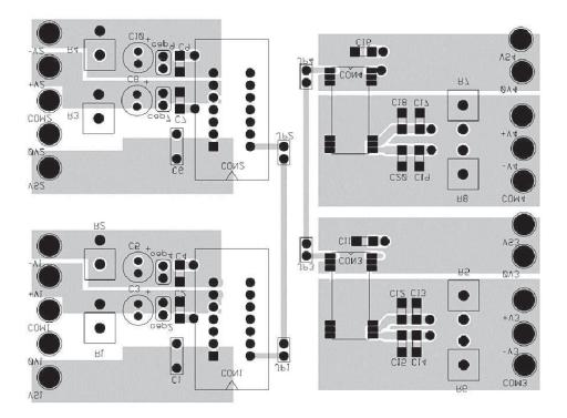
Figure 39. PCB Layout Example, Non-Component-Side View
