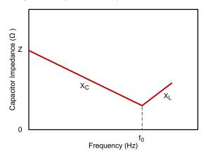
Figure 35. Capacitor Impedance vs Frequency
