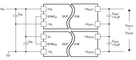
Figure 29. Multiple DCP01B Devices Connected in Series
