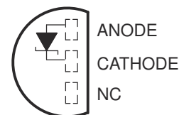
1.2 V . . . LP (TO-92/TO-226) PACKAGE (TOP VIEW)
