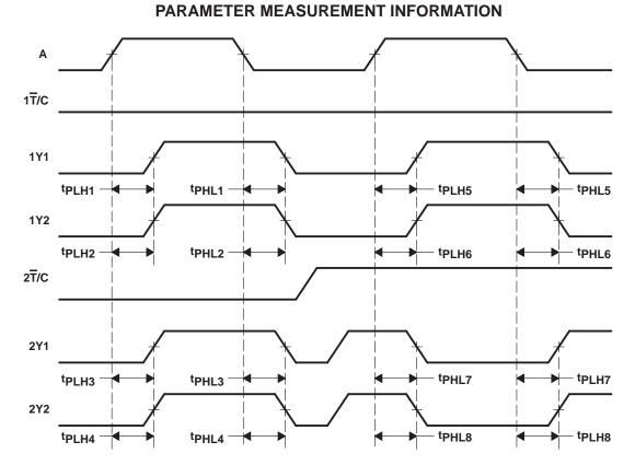
NOTES: A. Output skew, t<sub>sk(0)</sub>, from A to any Y (same phase), can be measured only between outputs for which the respective polarity-control inputs (T/C) are at the same logic level. It is calculated as the greater of:
