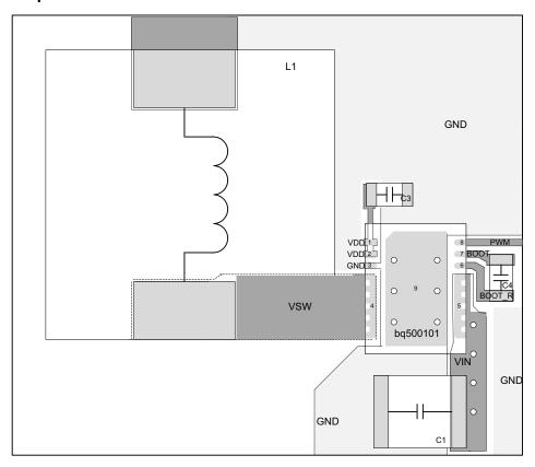
Figure 12. Recommended PCB Layout (Top Down View)
