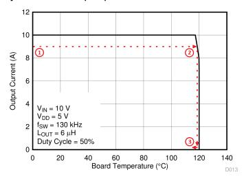
Figure 11. Power Stage bq500101 SOA, T<sub>A</sub> = 25°C
