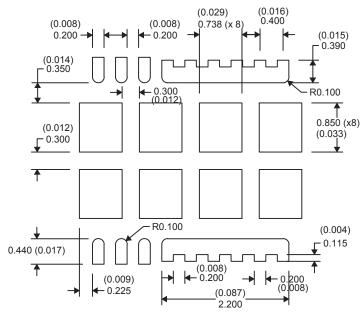
NOTE: Dimensions are in mm (inches). Stencil is 100  $\mu$ m thick.
