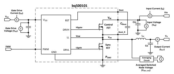
Figure 10. Power Loss Test Circuit
