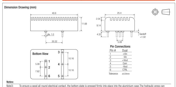
leave tooling marks and deformations to both the case and plate. The case is anodised aluminium, so there will be natural variations in the case colour and the aluminium is not scratch resistant. Any resultant marks, scratches and colour variations are cosmetic only and do not affect the operation or performance of the converters.
