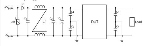
It is recommended to add UR1, D1 and C1 in railway application. C1, L1, C2 and C3 can be modified for required EMI standards. To meet EN61000-4-2, module case should be earth grounded. We offer independent case pin option on request.
