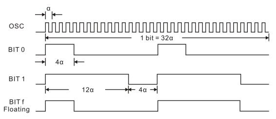
where: α=Oscillating Clock Period. Bit 1 is only available for Address Bit.
