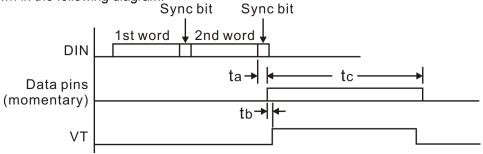
Note: ta=8 OSC clock width tb=1 OSC clock width tc=2 code word width
