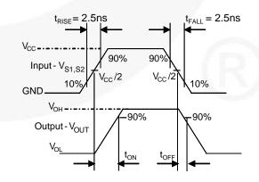
Figure 10. Turn-On / Turn-Off Waveforms
