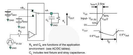
Figure 11. Break-Before-Make Timing
