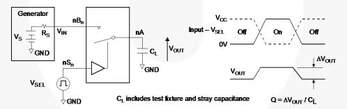
Figure 14. Charge Injection Test
