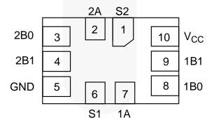
Figure 2. Pin Configuration
