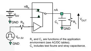
Figure 4. Test Circuit Load
