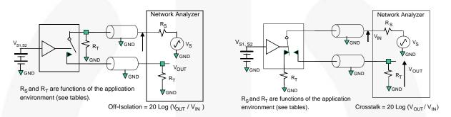
Figure 12. Channel Off Isolation
