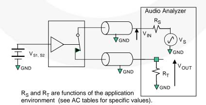
Figure 15. Total Harmonic Distortion
