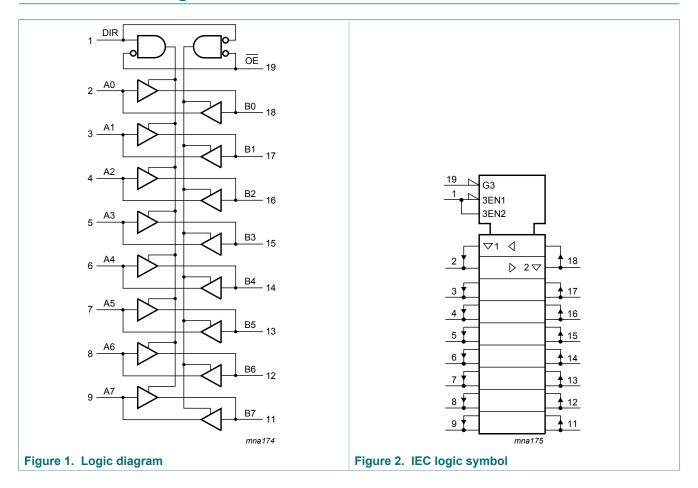
Octal transceiver with direction pin; 3-State
