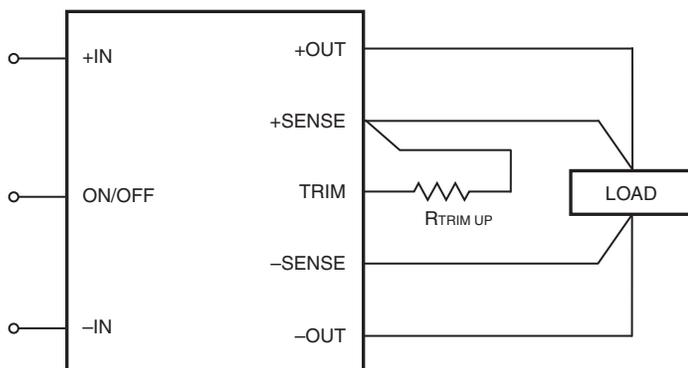
Figure 6. Trim Connections to Increase Output Voltages
