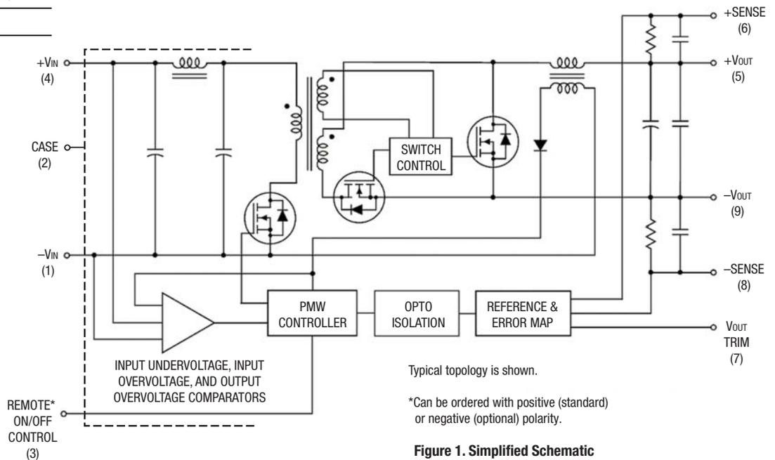
Figure 1. Simplified Schematic
