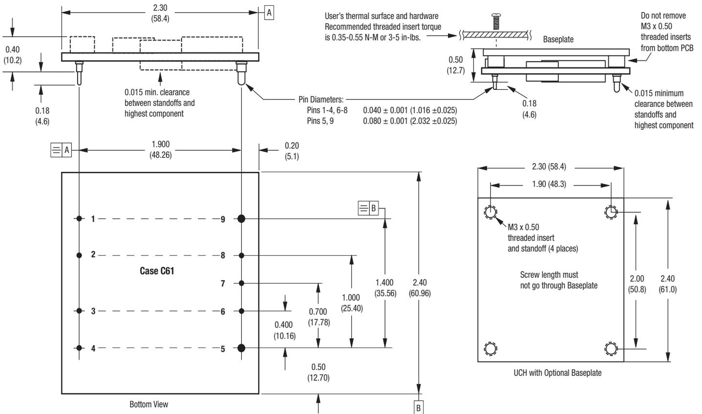
Standard pin length is shown. Please refer to the Part Number Structure for special order pin lengths.
