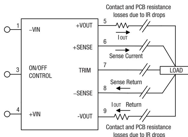
Figure 4. Remote Sense Circuit Configuration
