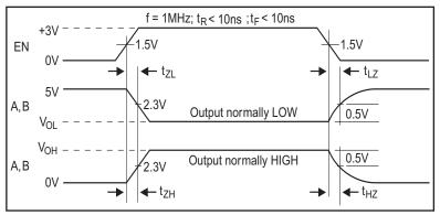
Figure 5. Driver Enable/Disable Timing
