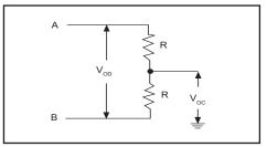
Figure 1. Driver DC Test Load
