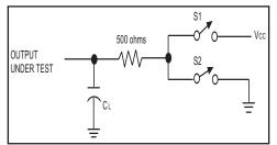
Figure 3. Driver Timing Test Load
