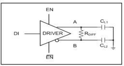
Figure 2. Driver Timing Test
