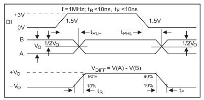
Figure 4. Driver Propagation Delays
