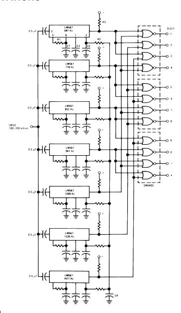
Component values (typ) R1 6.8 to 15k R2 4.7k R3 20k C1 0.10 mfd C2 1.0 mfd 6V C3 2.2 mfd 6V C4 250 mfd 6V
