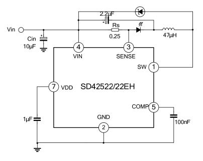
$6{\sim}36V$  input voltage, 350mA output LED driver
