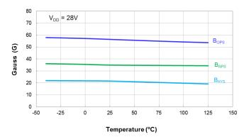
Switch Points B<sub>OPS</sub> and B<sub>RPS</sub> vs Temperature
