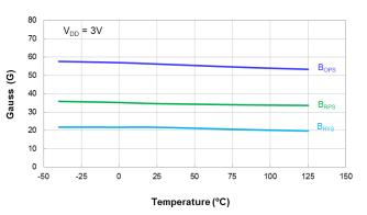
Switch Points  $B_{\text{OPS}}$  and  $B_{\text{RPS}}$  vs Temperature
