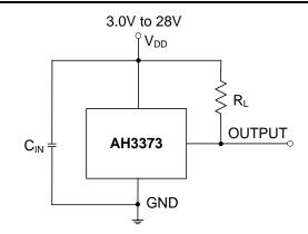
Note: 4.  $C_{IN}$  is for power stabilization and to strengthen the noise immunity, the recommended capacitance is 10nF ~ 100nF. R<sub>L</sub> is the pull-up resistor.
