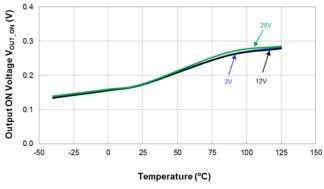
**Output ON Voltage vs Temperature**
