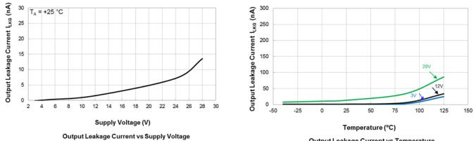
**Output Leakage Current vs Temperature**
