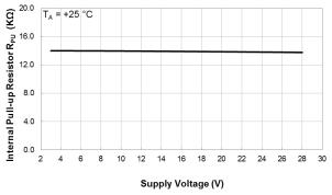
Internal Output Pull-up Resistor vs Supply Voltage
