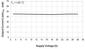
Output Current Limit vs Supply Voltage
