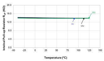
Internal Output Pull-up Resistor vs Temperature
