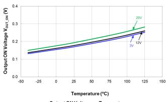
Output ON Voltage vs Temperature
