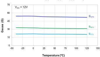
Switch Points B<sub>OPS</sub> and B<sub>RPS</sub> vs Temperature
