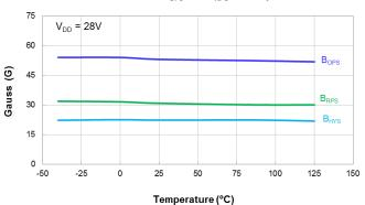
Switch Points  $\mathbf{B}_{\text{OPS}}$  and  $\mathbf{B}_{\text{RPS}}$  vs Temperature
