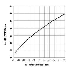
Figure 4: Typical HFBR-14x4xZ/HFBR-24x2xZ Link with 62.5/125 µm Fiber
