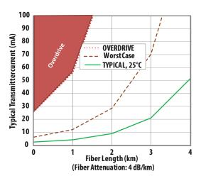
Figure 5: Typical HFBR-14x4xZ/HFBR-24x2xZ Link with 50/125  $\mu m$  Fiber
