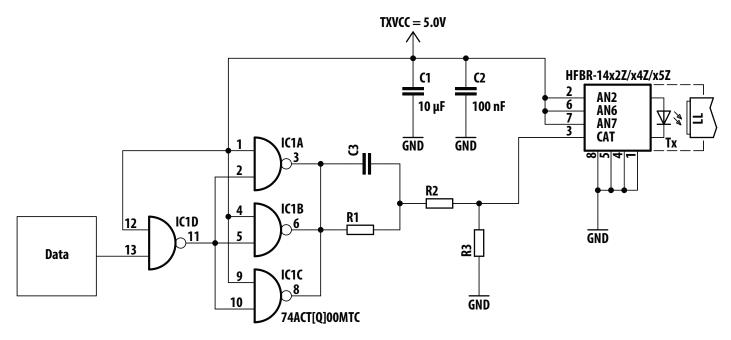
**NOTE:** The component values shown in the table create a typical driver current of 60 mA (peak). An individual check of the optical output signal quality of the used optic transmitter is recommended during the circuit design.
