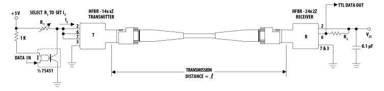
**NOTE:** A bypass capacitor (0.01 µF to 0.1 µm ceramic) must be connected from pin 2 to pin 7 of the receiver. Total lead length between both ends of the capacitor and the pins should not exceed 20 mm.
