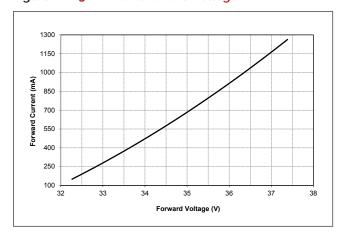
Figure 3: V13B Drive Current vs. Voltage
