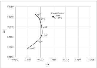
Figure 13: 3500K Class A Color Shift vs. Case Temperature<sup>1</sup>
