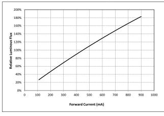
Figure 4: V13C Typical Relative Flux vs. Current
