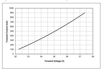
Figure 2: V13C Drive Current vs. Voltage
