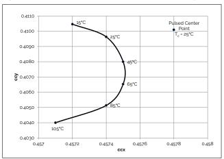
Figure 12: 3000K Class A Color Shift vs. Case Temperature<sup>1</sup>
