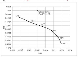
Figure 10: 2700K, 97 CRI Color Shift vs. Case Temperature<sup>1</sup>
