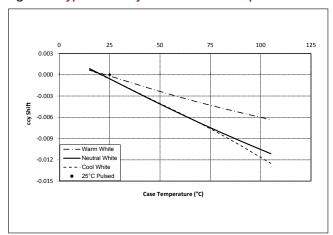
Figure 7: Typical DC ccx Shift vs. Case Temperature
