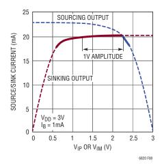
Figure 8. Drive Source/Sink vs Output Voltage
