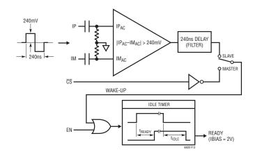
Figure 13. Wake-Up Detection and IDLE Timer
