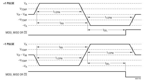
Figure 2. isoSPI Differential Pulse Detail
