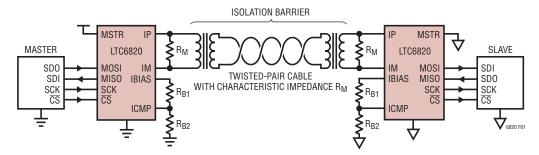
Figure 1. Typical System Using Two LTC6820 Devices
