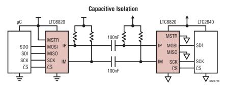
Figure 18. Capacitive Isolation Barrier
