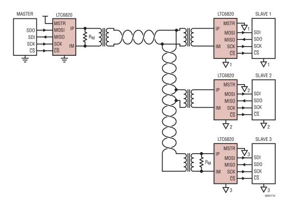
Figure 16. Multidropping Multiple Slaves on a Single Cable
