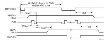
Figure 15. Master and Slave Wake-Up/Idle Sequence
