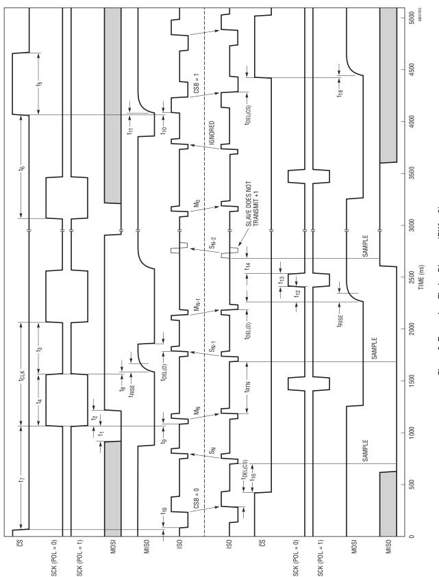
Figure 3. Transceiver Timing Diagram (PHA =  $\mathbf{0}$ )
