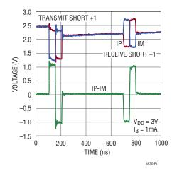
Figure 11. Transmitting and Receiving Data
