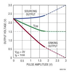
Figure 9. Output Voltages and Common Mode vs Amplitude
