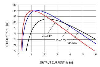
Figure 1. Converter Efficiency versus Output Current.
