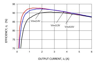
Figure 13. Converter Efficiency versus Output Current.
