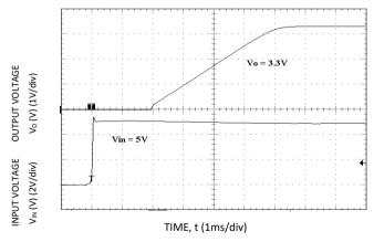
Figure 30. Typical Start-up Using Input Voltage ( $V_{IN} = 5V$ ,  $I_0 = I_{0,max}$ ).
