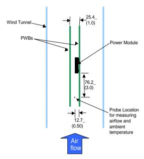
Figure 45. Thermal Test Setup.
