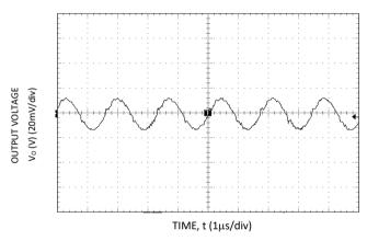
Figure 15. Typical output ripple and noise ( $V_{IN} = 5V$ ,  $I_0 = I_{O,max}$ ).
