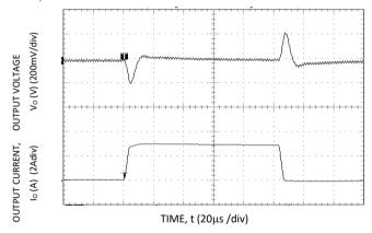
Figure 28. Transient Response to Dynamic Load Change from 0% 50% to 0% with  $V_{\text{IN}}$ =5V.
