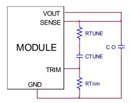
Figure. 44. Circuit diagram showing connection of  $R_{\text{TUME}}$  and  $C_{\text{TUNE}}$  to tune the control loop of the module.
