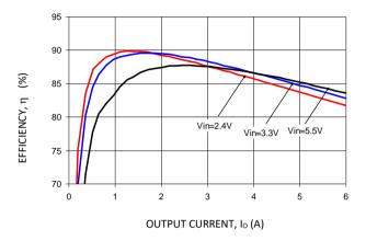
Figure 7. Converter Efficiency versus Output Current.
