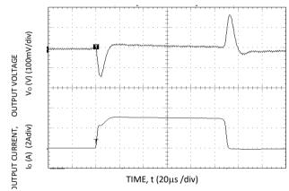
Figure 4. Transient Response to Dynamic Load Change from 0% to 50% to 0% with  $V_{\text{IN=5V}}$  .
