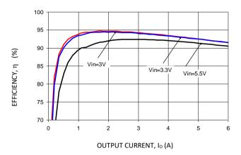
Figure 19. Converter Efficiency versus Output Current.
