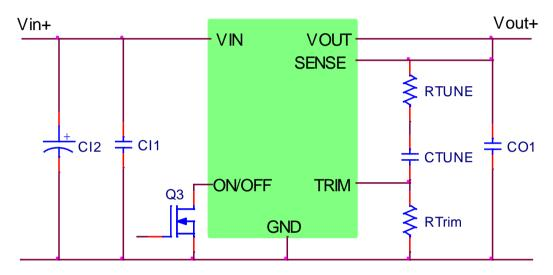
CIN1  $2 \times 22\mu F/6.3V$  ceramic capacitor CIN2  $47\mu F/6.3V$  bulk electrolytic
