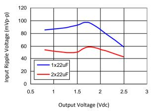
Figure 35. Input ripple voltage in mV, p-p for various output voltages with 1x22  $\mu$ F or 2x22  $\mu$ F ceramic capacitors at the input (6A load). Input voltage is 3.3V.
