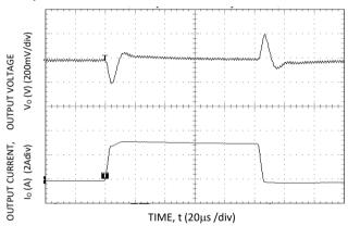
Figure 22. Transient Response to Dynamic Load Change from 0% to 50% to 0% with  $V_{\rm IN}$ =5V.
