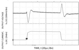
Figure 16. Transient Response to Dynamic Load Change from 0% to 50% to 0% with  $V_{\text{IN}}$ =5V.
