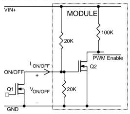
Figure 38. Circuit configuration for using positive On/Off logic.
