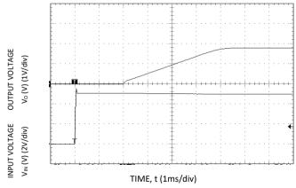
Figure 18. Typical Start-up Using Input Voltage ( $V_{IN} = 5V$ ,  $I_0 = I_{O,max}$ ).
