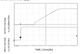
Figure 6. Typical Start-up Using Input Voltage ( $V_{IN} = 5V$ ,  $I_0 = I_{O,max}$ ).
