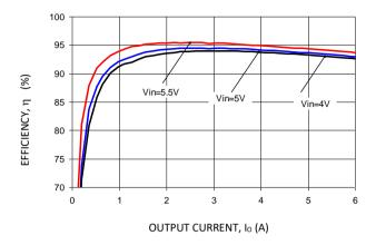
Figure 25. Converter Efficiency versus Output Current.
