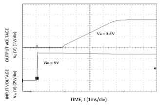
Figure 24. Typical Start-up Using Input Voltage ( $V_{IN}$  = 5V,  $I_0$  =  $I_{0,max}$ ).
